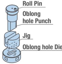
\*TA99037 Lock Nut Ass'y is required for Oblong hole D Punch 25 x 9 / 12 / 14 / 18
